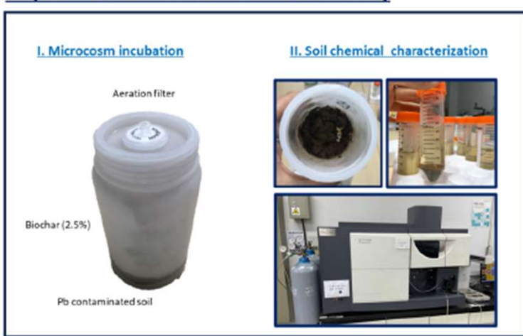
Fig. 1 An overall framework proposed to address the objective of determining the effectiveness of Pb immobilization with biochar
